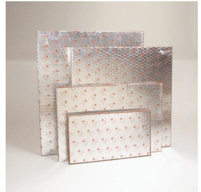
The nominal 0.3" (7.62 mm) thick composite sheet provides up to a 4-hour fire rating when properly installed. It is lightweight and can be easily installed with common trade tools. When exposed to temperatures in excess of 250°F (121°C), the fire-resistive sheet begins to volumetrically expand and swells 8–10 times its original size, forming a high strength, hard char that retards heat transmission.
