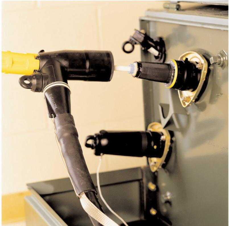
wire shield, UniShield® and jacketed concentric neutral types of cable. 3M's elbows are molded using high quality peroxide-cured EPDM insulation and meet requirements of ANSI/IEEE Standard 386.
